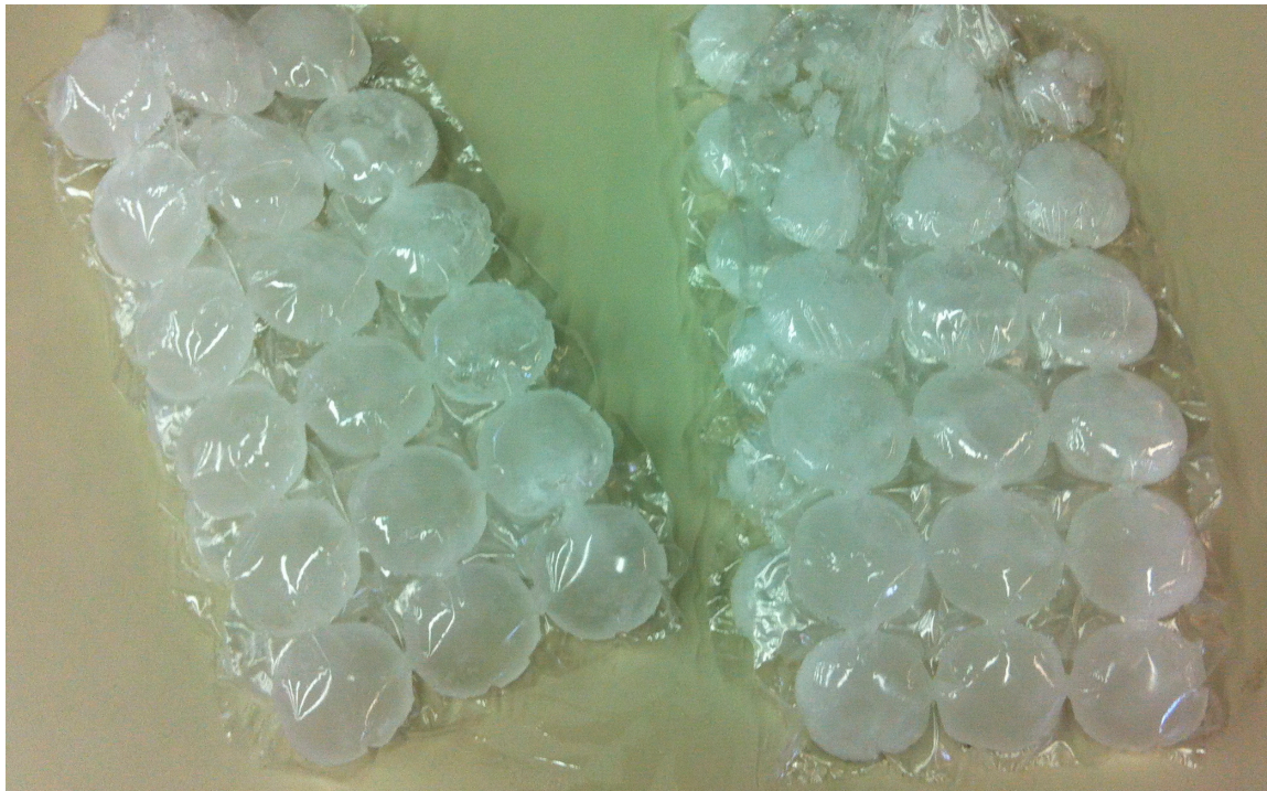
Figure 2. Paraffin-based phase change material (PCM) encapsulated in plastic discs.
