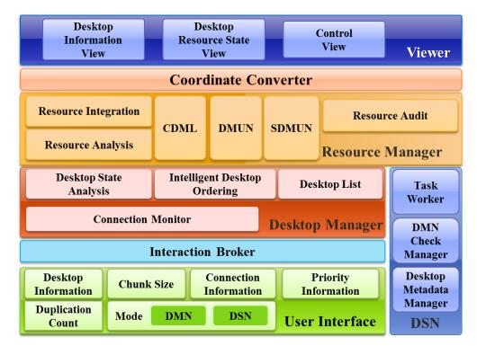
**Figure 3.** Sustainable Operation System for Integrated desktop Resources (SOSIDR) Architecture for Sustainable Operation.
