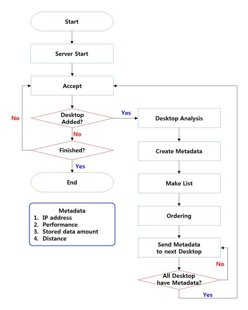
Figure 1. Desktop Master Node (DMN) flow for sustainable operation.
