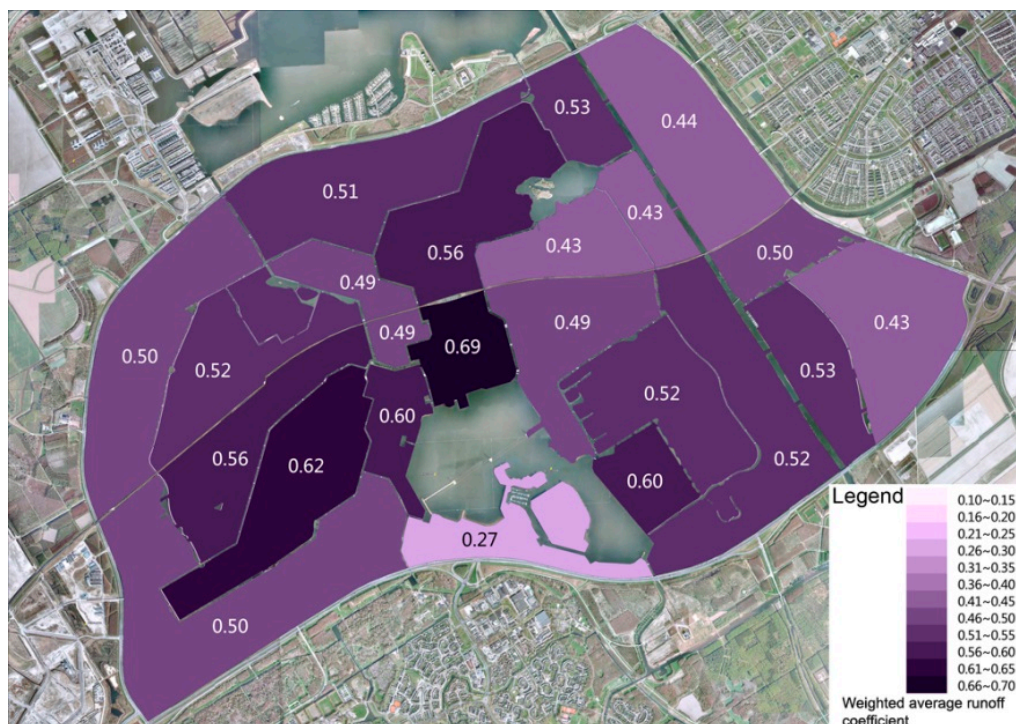
Figure 9. Weighted average runoff coefficient of each block in Almere Stad.
