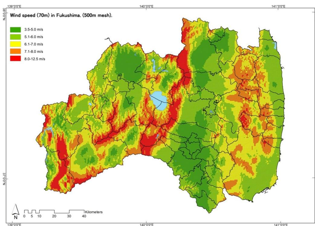
GIS resources used were Fukushima municipal boundary, topography, designated areas, and land use datasets, the same we used for solar potential estimation in Section 5.2.1. Wind speed data (in the form of “.dat” files, converted to GIS mesh polygon as mentioned above) and their annual occurrence frequency (bar graph) were obtained from the local area wind energy prediction system provided by New Energy and Industrial Technology Development Organization (NEDO) [63].
