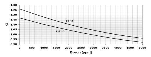
Figure 4. Ke as a function of boron concentration.
