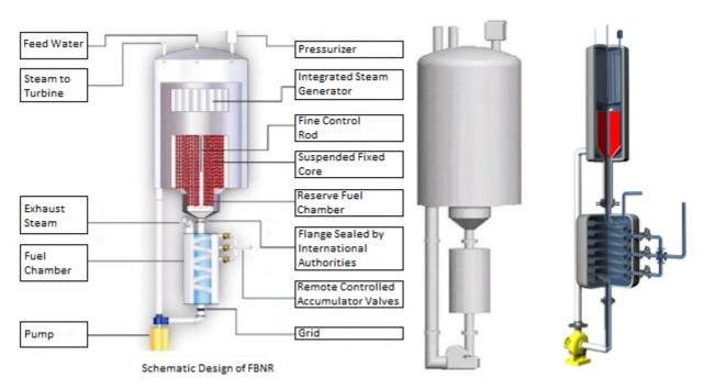
Figure 1. Schematic Design of the Fixed Bed Nuclear Reactor (FNBR).
