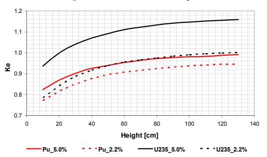
Figure 8. Ke as a function of core height.
