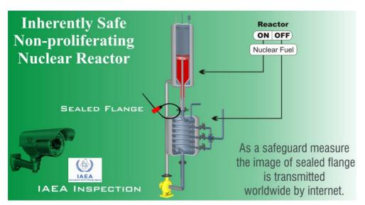
Figure 3. Schematic figure of inherently safe non-proliferating nuclear reactor.
