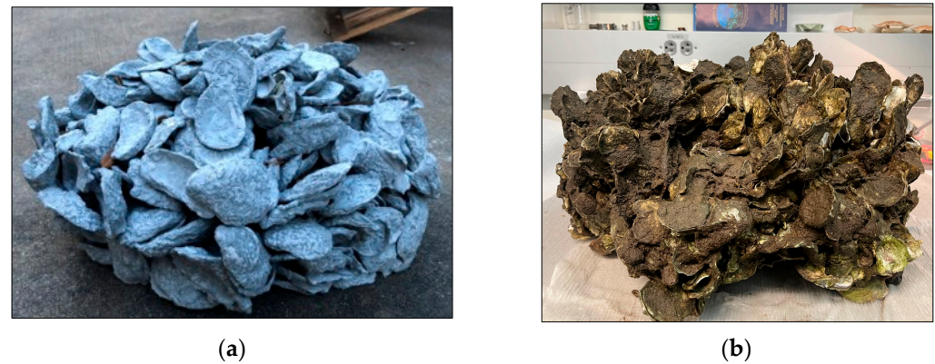
Figure 1. Typical POSH module (a) prior to deployment and (b) two years post-deployment at Kingsley Plantation along the Fort George River.
