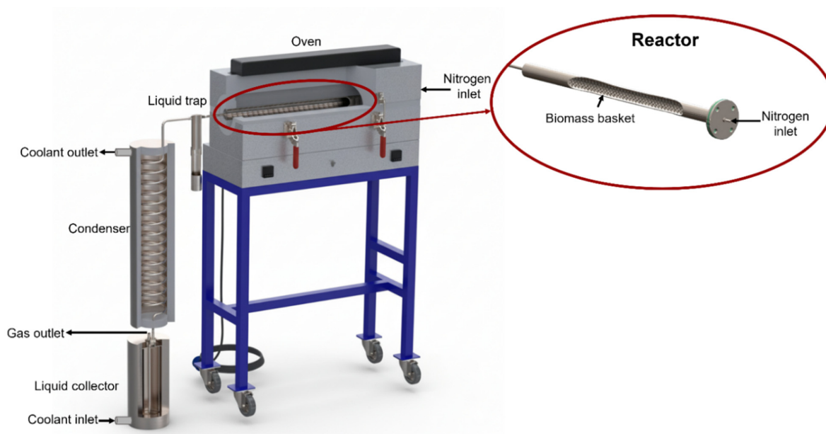
Figure 1. Schematic representation of the biomass pyrolysis system.
