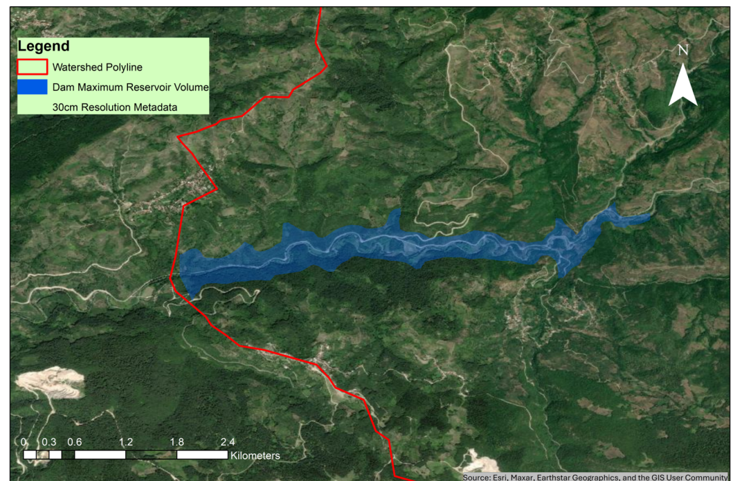
Figure 7. Spatial mapping of the peak reservoir inundation limits at the designated 466 m crest height, integrated with 30 cm resolution satellite datasets, to evaluate the projected environmental footprint across the local terrain.
