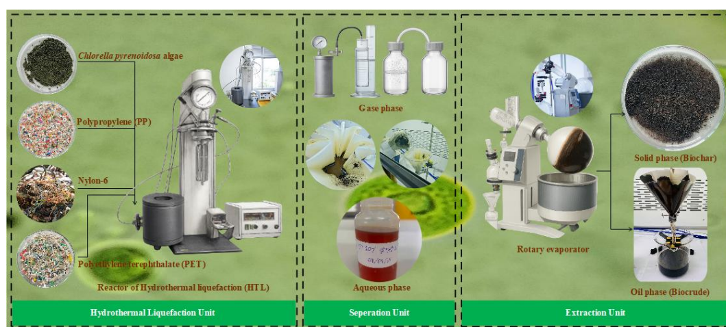
Figure 2. Schematic representation of the co-hydrothermal liquefaction process of Chlorella pyrenoidosa algae and post-recycling plastic wastes, showing hydrothermal liquefaction, separation, and extraction units with corresponding product phases.
