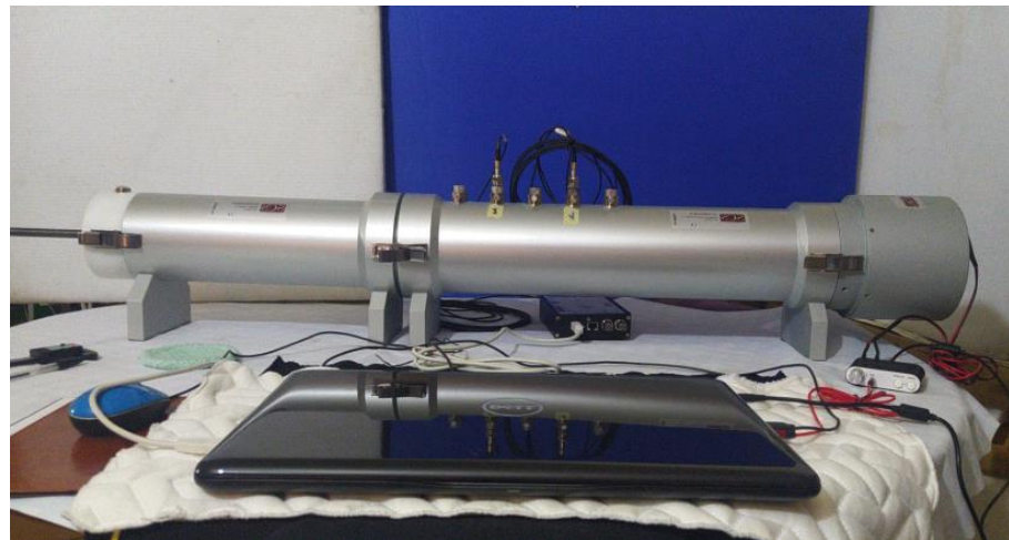
Figure 3. Impedance tube used for measuring the normal-incidence sound absorption coefficient (Model SCS, Type 9020B/K).
