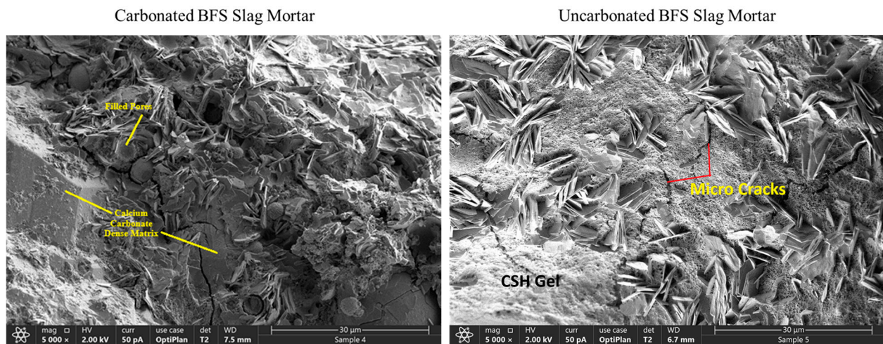
Figure 13. Microstructure Analysis of Mortar Samples from Uncarbonated and Carbonated BFS Slag Aggregates.
