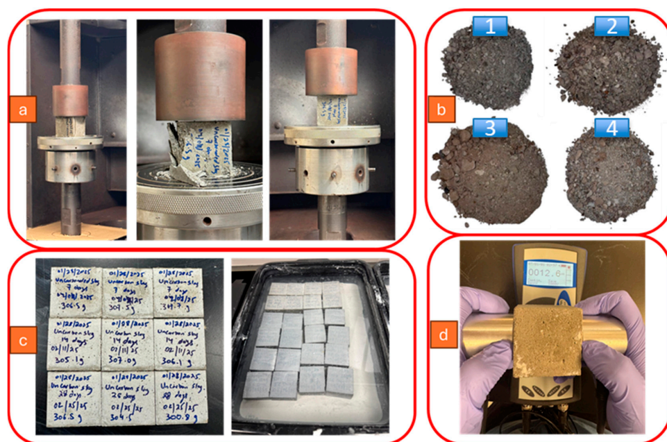
Figure 3. Summary of experimental procedures and materials. (a) Compressive strength testing of mortar samples using MTS. (b) Standard water curing of mortar cubes at 7, 14, and 28 days. (c) Visual representation of the four slag types used as aggregates: (1) Rockport slag, (2) Skim slag, (3) BOF slag, and (4) Blast furnace slag. (d) UPV Testing.
