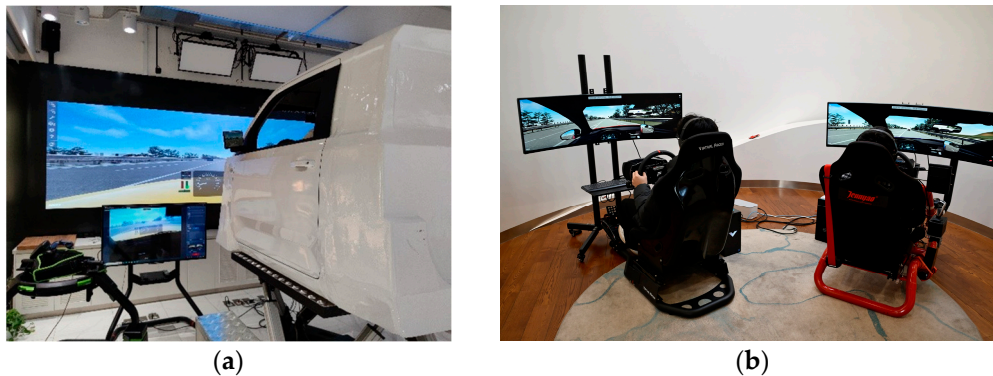
Figure 6. Experimental Process: (a) Experimental Process of the Six Degrees of Freedom Driving Simulator; (b) Experimental Process of the Fixed Base Driving Simulator.
