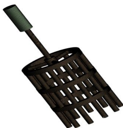
Figure 14. Mesh model of the lateral rotary-type soil cleaning device.
