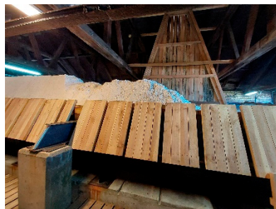
Figure 7. Drying the salt on the boards above the bathtub (S. Chudy).
