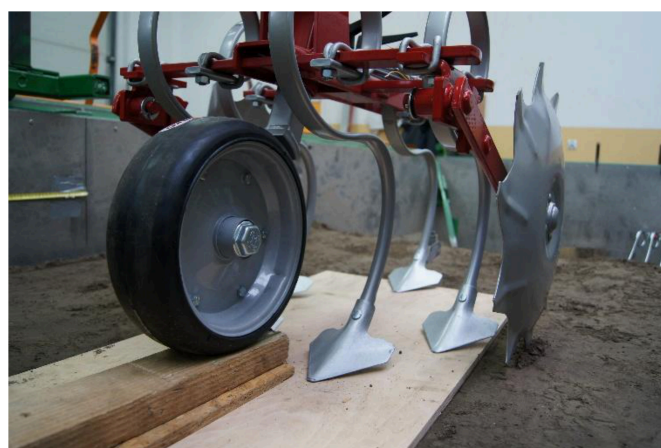
Figure 2. View of the weeding section equipped with three duckfoots and two shields covering the rows of plants (shows how to set the working depth).
