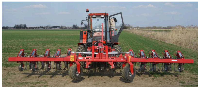
Figure 1. Mounted in-line cultivator at the front of a tractor, prepared for field testing.
