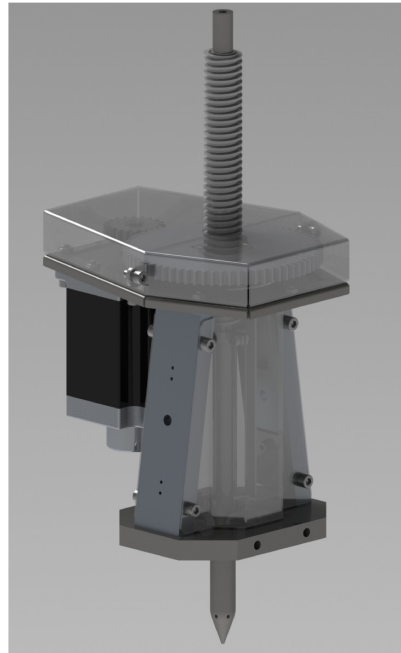
Figure 2. Three-dimensional model of pressurized steam injection system.
