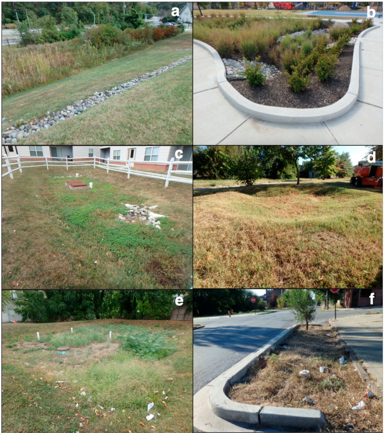
Figure 3. Examples of regulatory (a,c,e) and voluntary (b,d,f) GSI facilities with different scores and characteristics. GSI facilities shown in (a,b) received high scores, while those in (e,f) received low scores. GSI facilities in (c,d) had intermediate scores due to good maintenance, although they lack vegetation complexity and clear aesthetic design elements.
