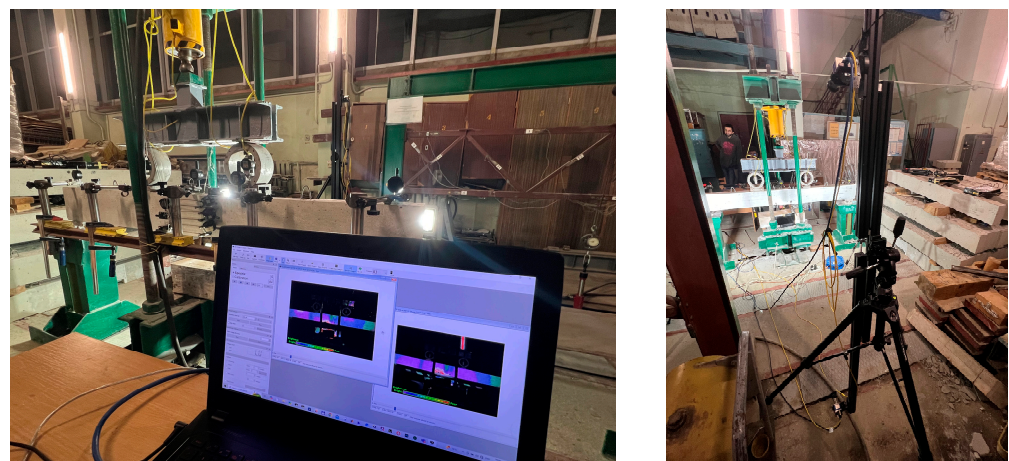
Figure 3. An example of using digital image correlation for determining strains and deflections of reinforced concrete structures (authors' own research).
