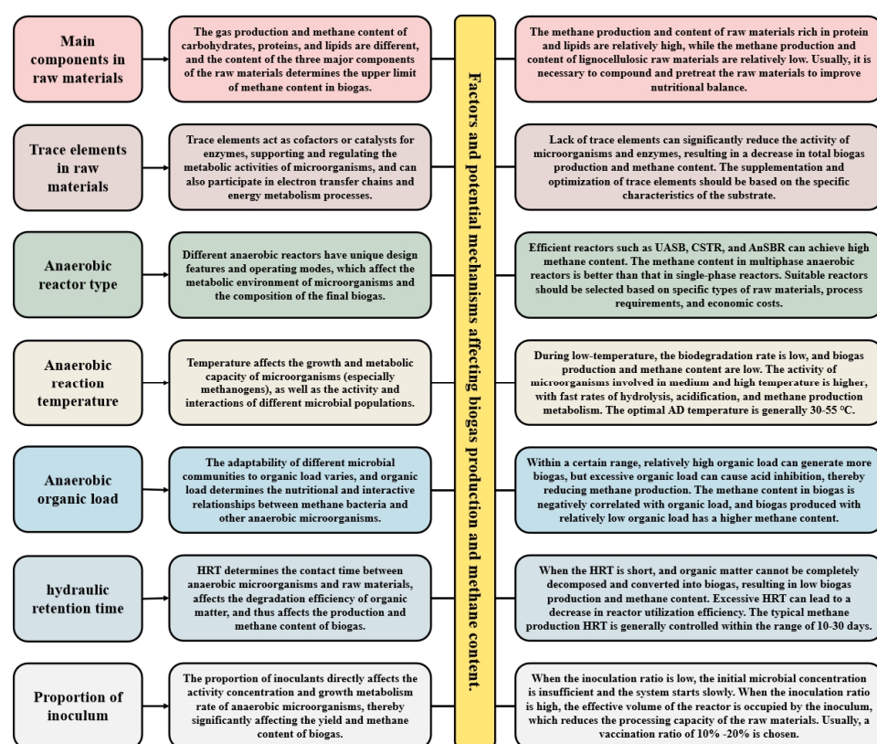
Figure 2. The factors affecting CH 4 content in biogas during AD process.
