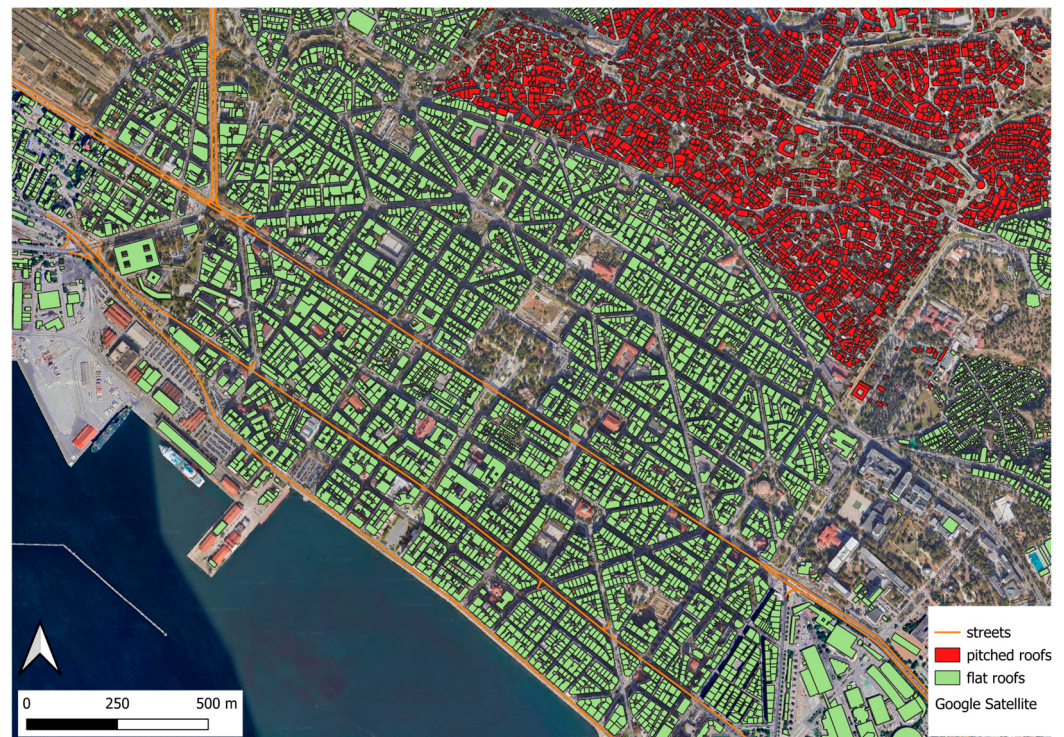
Figure 8. Rough general overview of potential flat roofs that can be converted into green roofs (flat roofs), with the old town lacking similar structures (pitched roofs) (Source: Authors with QGIS).
