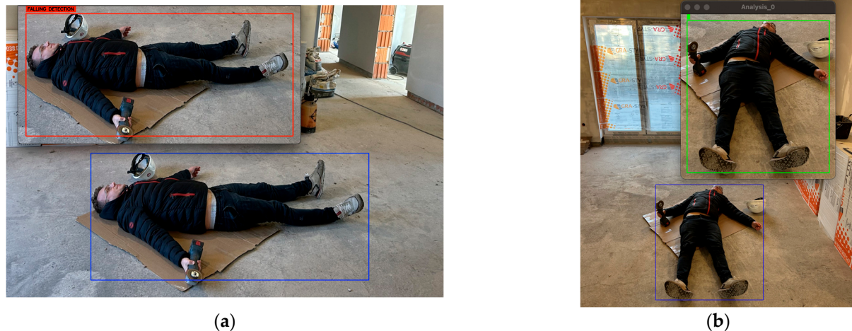
Figure 7. Analysis of the event detection system in the human fall category: (a) Correct event detection; (b) Failure to detect a human fall, even though an accident occurred.
