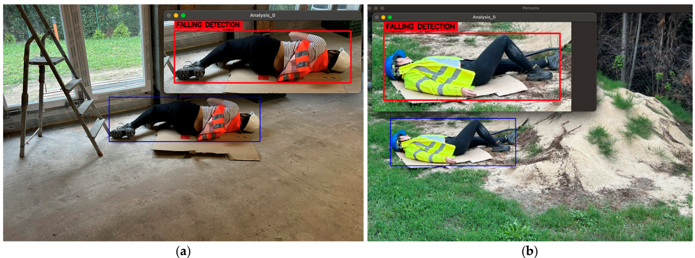
Figure 6. Video output frames showing the expected classification change in the event of a human fall detection: (a) scene from an outdoor construction site; (b) scene from an outdoor construction site.
