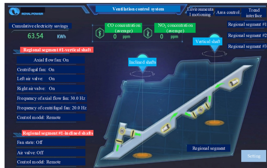
Figure 3. A typical PLC in the tunnel ventilation system (the green arrow represents the direction of the airflow).
