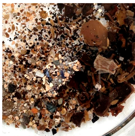
Figure 16. Settled contaminants from biowaste samples in the fiber after TPH for paper production.
