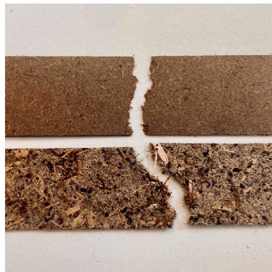
Figure 19. Sheet structure and fracture edge (top: cup-plant; bottom: biowaste).
