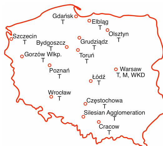
Figure 4. Rail urban and suburban electrified systems in Poland (T—trams, M—metro, WKD—suburban railway transport).
