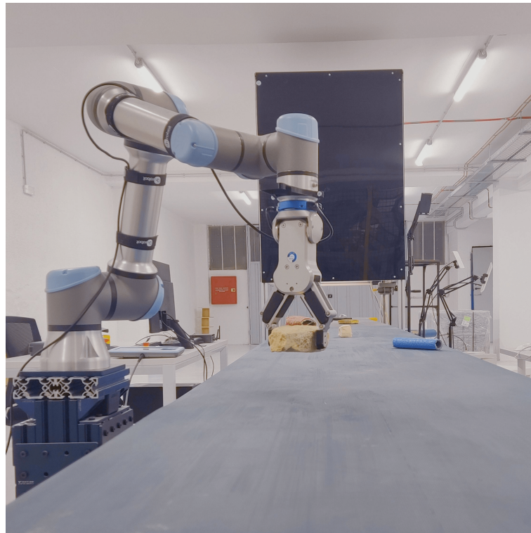
Figure 9. UR5e Robot, finger gripper, and conveyor performing CDW sorting experiments.
