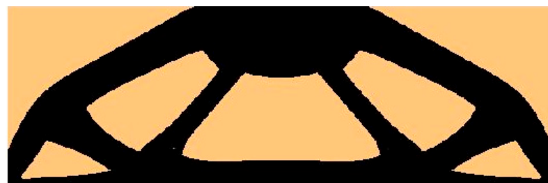
Figure 8. The final topology for the structure under a single deterministic load.
