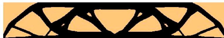
Figure 13. The final topology for the structure under a single deterministic load.
