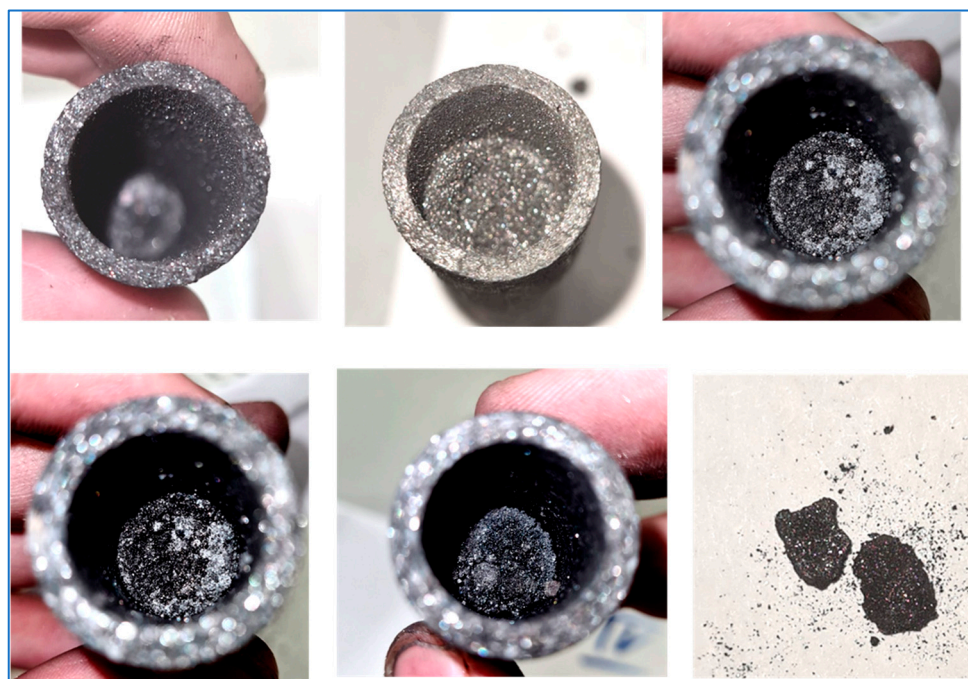
Figure 1. Representative examples of heat-treated RM and its blends after carbothermic reduction at 1650 °C for 20 min.
