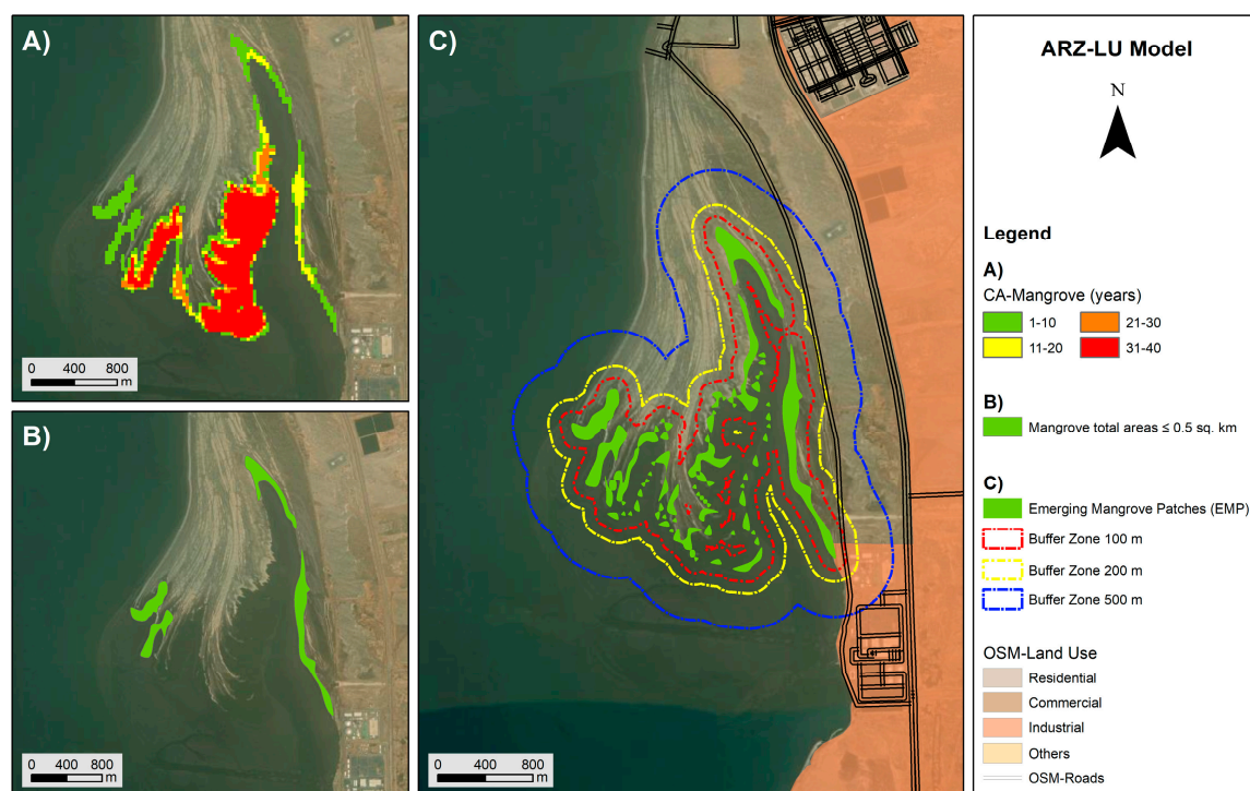
Figure 9. At-risk zones based on land use and transportation networks. (A) chronological age of mangrove areas over 40 years; (B) The vulnerable mangrove areas less than or equal to 0.5 km 2 ; and (C) the At-Risk Zones Based Land Use (ARZ-LU) model.
