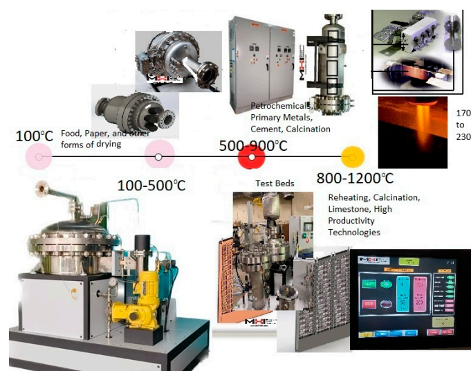
Figure 1. The gamut of heating process temperatures from 100 °C to 1200 °C, with typical applications in the industrial sector (picture provided by MHI Inc., Cincinnati, OH, USA, reproduced with permission). From left to right, the pictures show electrical steam generation, electrical process gas heating, logic control displays, and the EION system discussed in Section 4.
