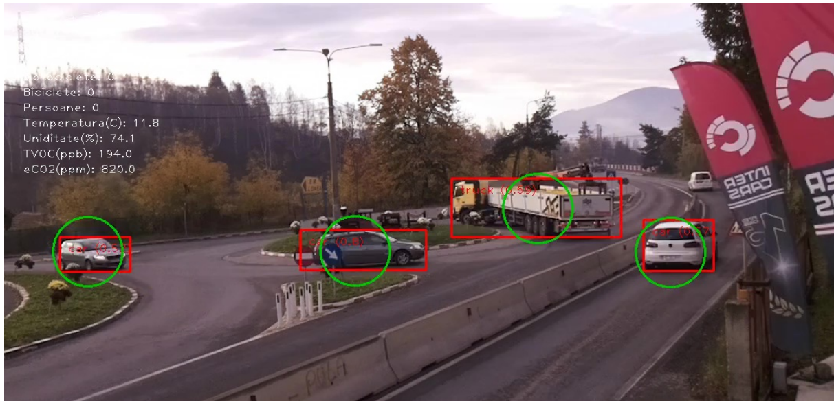
Figure 12. Captured frame with overlays showing vehicle detection at location 3, red box and green circle indicating detection by the counter algorithm.
