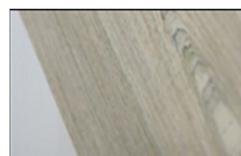
Figure 6. Wood material made from newspapers. Material made from old newspapers pressed together using non-water-based glue. It is a sustainable alternative to wood, is lightweight, and is used in furniture pieces.
