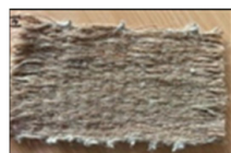
Figure 4. Raw material of date palm fibers. Date palm fiber fabric panels, a sustainable local material, enhance the sound absorption quality of interior spaces [29].
