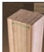
Figure 5. Raw material of date palm frond waste. A handmade material made by cutting palm frond branches into long pieces, then drying them and cutting them into pieces of equal length. These pieces are assembled, glued together, and used as an alternative to imported wood.
