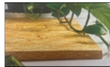
Figure 3. Natural-straw fiberboards. Made from 100% straw, it is used in interior applications such as furniture making and interior construction and is characterized by being treated with organic waste [28].
