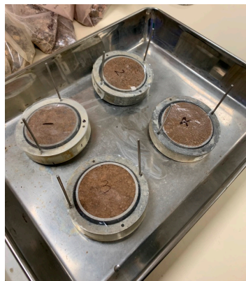
Figure 7. Specimen for centrifuge test.
