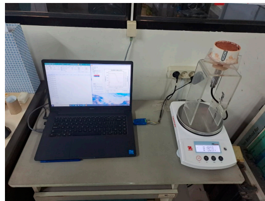
Figure 6. SWCC test by using PBT.
