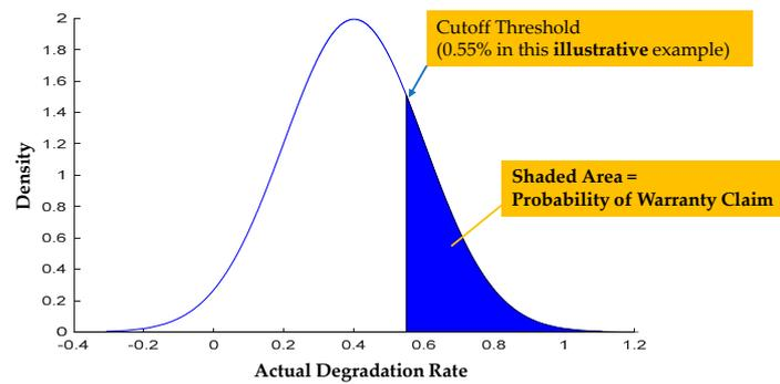
**Figure 4.** Illustration example for deriving probability of claim and expected shortfall
