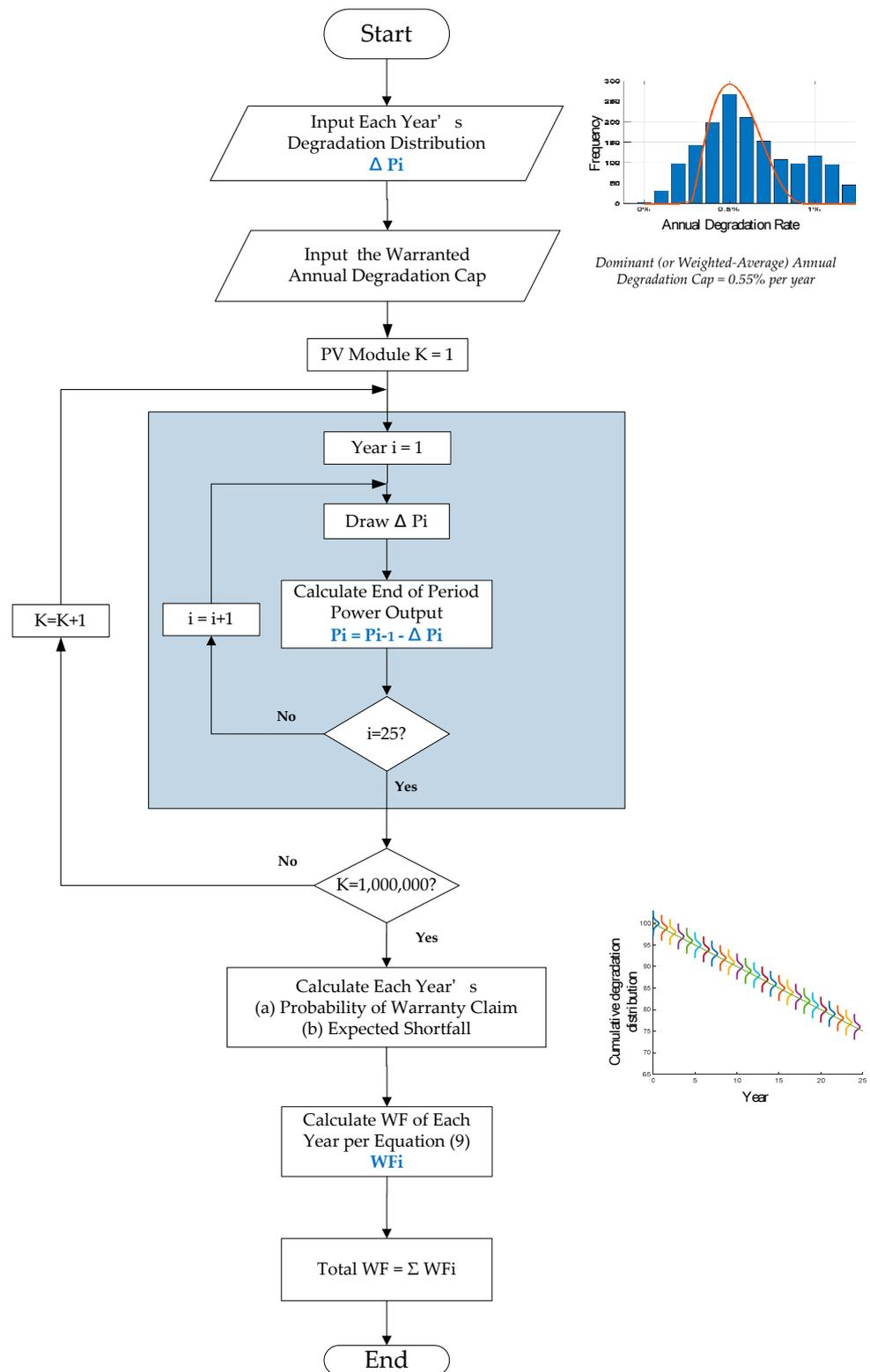
Figure 5. Monte Carlo simulation procedure used in this study
