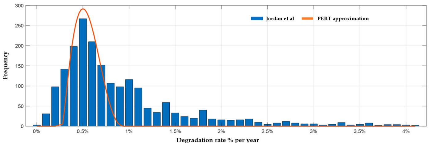
**Figure 3.** Benchmark PV degradation rate distribution and PERT approximation.
