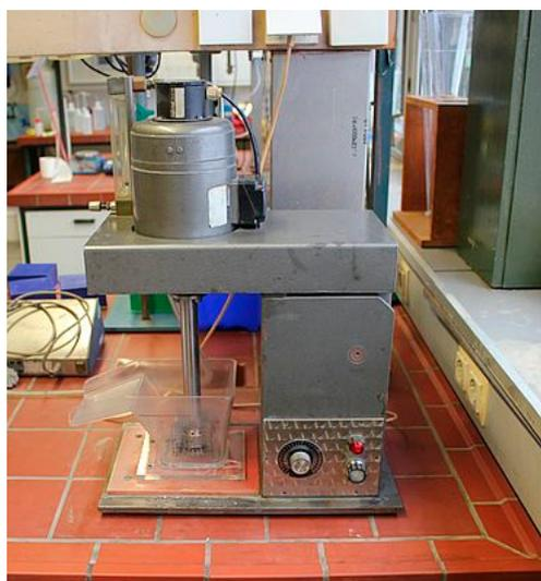
**Figure 2.** IFAD-construction Denver-type flotation machine (IA 0583/3).
