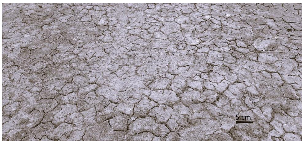
**Figure 1.** Network of desiccation cracks in fine-grained soil.
