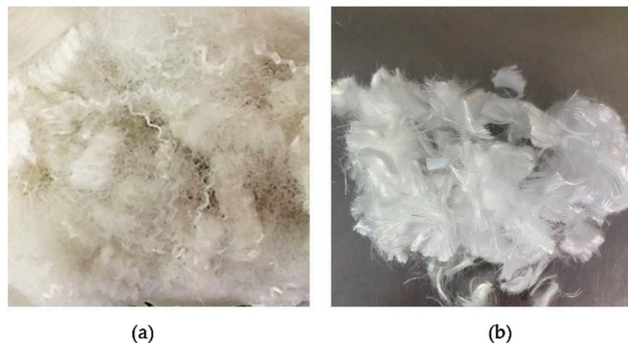
Figure 3. Recycled fibers used: (a) polyethylene terephthalate; (b) polypropylene.
