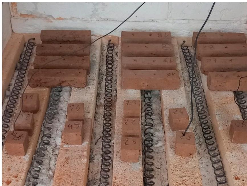
Figure 3. Samples during the firing process, with thermocouples visible.
