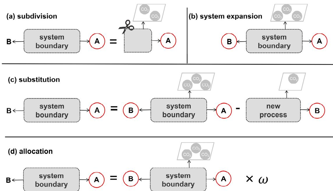
**Figure 1.** Schematic diagram of four methods of allocation (the red circle represents the functional unit).
