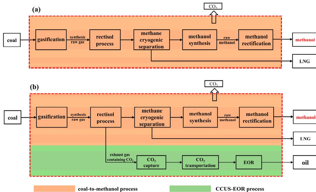
**Figure 2.** Boundary of the system to calculate the carbon footprint. (a) Scenario 1: not coupled with CCUS-EOR. (b) Scenario 2: coupled with CCUS-EOR.
