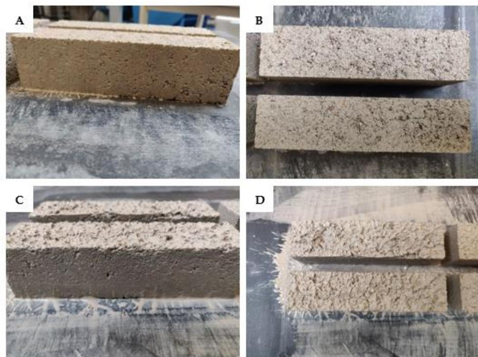
**Figure 15.** Mix 1 series of lab-phase examinations on prisms after vibropressing. (A) Mix 1/95/5/MC10% prism side view, (B) Mix 1/95/5/MC10% prism top view, (C) Mix 1/95/5/MC13% prism side view, (D) Mix 1/95/5/MC13% prism top view.
