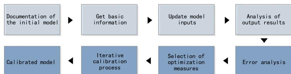
Figure 24. Process of model calibration method [45].
