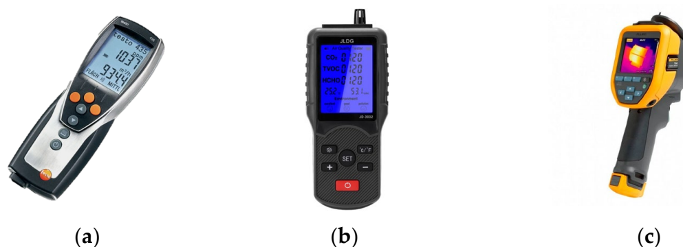
Figure 1. Equipment: (a) Testo 435. (b) JD-3002 air quality tester. (c) Fluke thermal camera.
