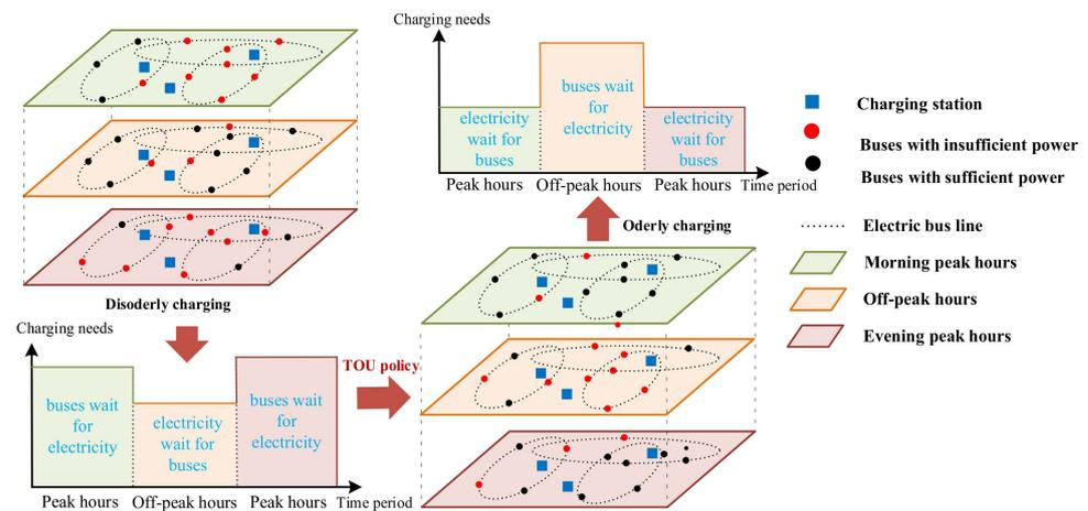
**Figure 2.** The charging system of EBs.
