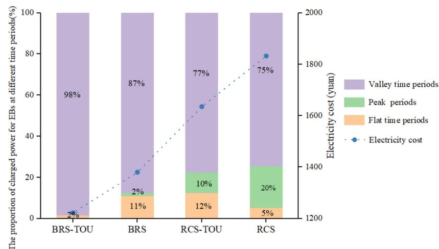
Figure 7. The electricity cost and the amount of recharged power.
