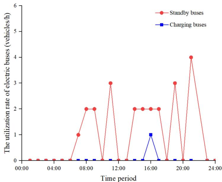
**Figure 5.** The number of bus replacements and charging times of standby buses.
