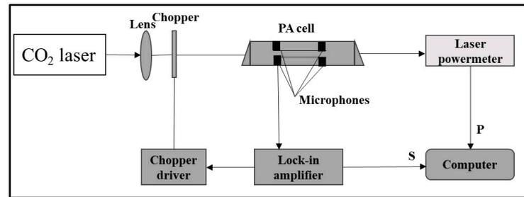
**Figure 1.** This diagram illustrates the laser photoacoustic setup used for trace gas measurements [31].
