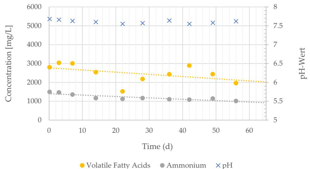
**Figure 9.** Chemical parameters during continuous operation.
