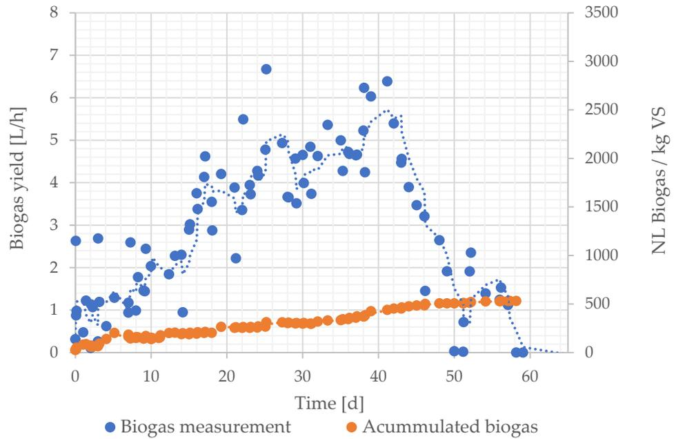
Figure 6. Biogas yield and specific biogas yield during normal continuous operation.
