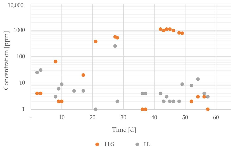
**Figure 8.** Presence of trace gases during normal operation.
