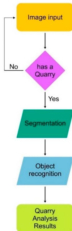
**Figure 1.** Workflow of the process developed for the aggregates quarry detection.
