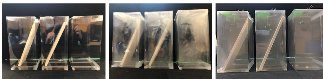
Figure 12. Sample boxes used in evaluating smoke removal: sample boxes (left), introduction of smoke (middle), smoke removal study after 10 min (right).
