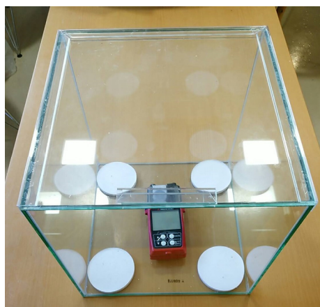
Figure 7. Formaldehyde adsorption study using circular gypsum boards.
