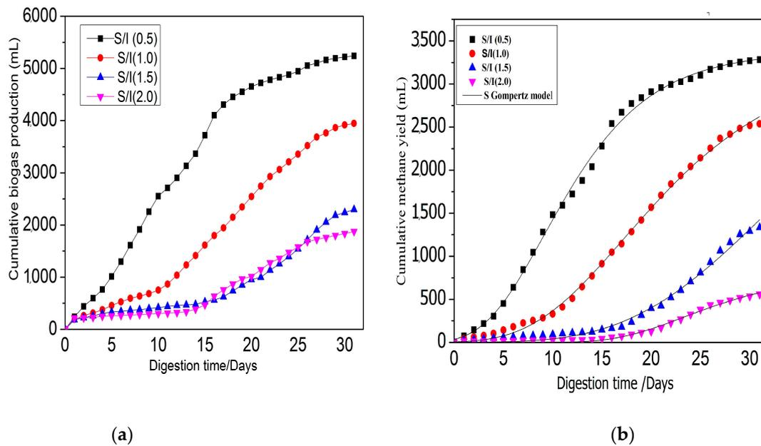
**Figure 3.** The cumulative biogas (a) and bio-methane production (b) for co-substrate mixtures at different S/I ratios.
