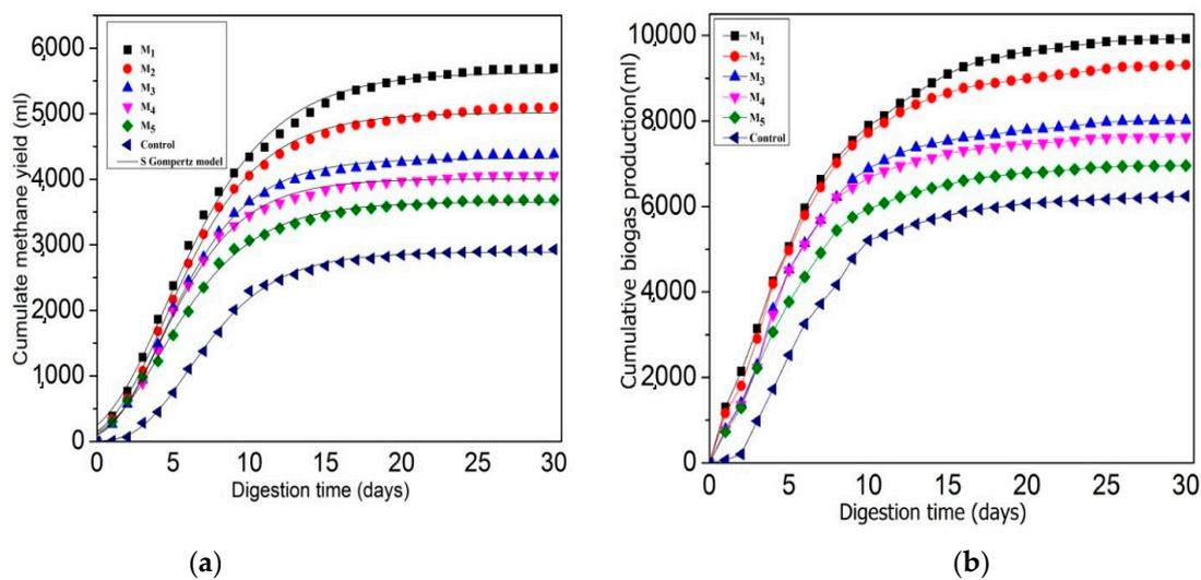
**Figure 2.** The cumulative bio-methane (a) and biogas yield (b) for co-substrate mixtures at different C/N ratios.
