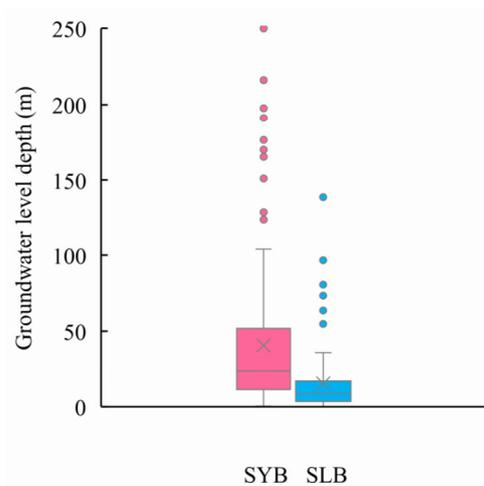
**Figure 3.** Box diagram of the groundwater level depth (GWD) in the Shiyang River Basin (SYB) and the Shule River Basin (SLB) of the Hexi Corridor. Boxes represent 25th, 50th, and 75th percentile values, and whiskers represent 10th and 90th percentile values. Scatter points represent extreme values.
