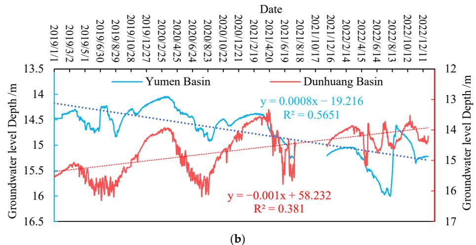
**Figure 4.** Daily variation of groundwater level depth in typical monitoring wells in the Hexi Corridor. (a) The Shiyang River Basin (SYB) and (b) the Shule River Basin (SLB).
