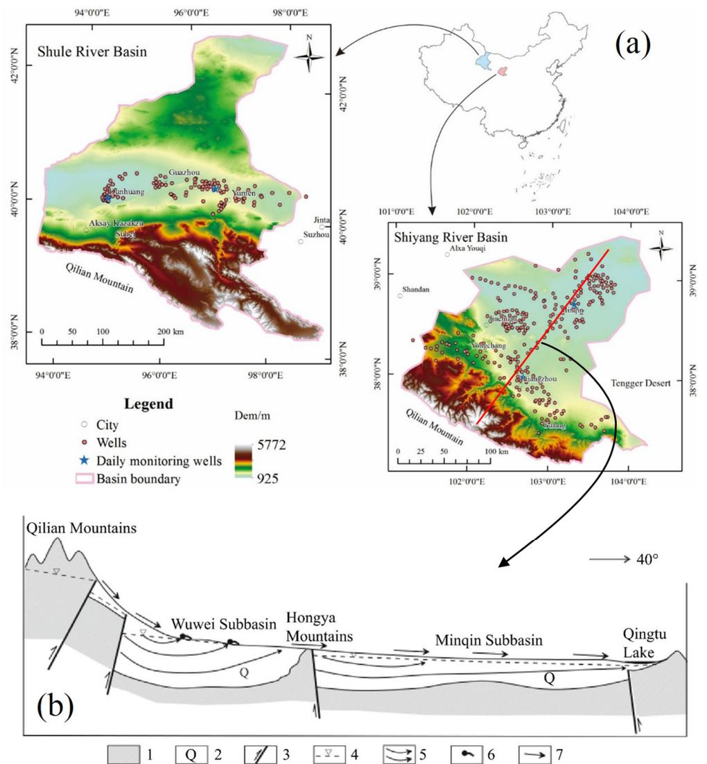
1-Bedrock; 2-Quaternary; 3-Fault; 4-Goudwater table; 5- Groundwater movement; 6-Spring; 7-Surface runoff flow
