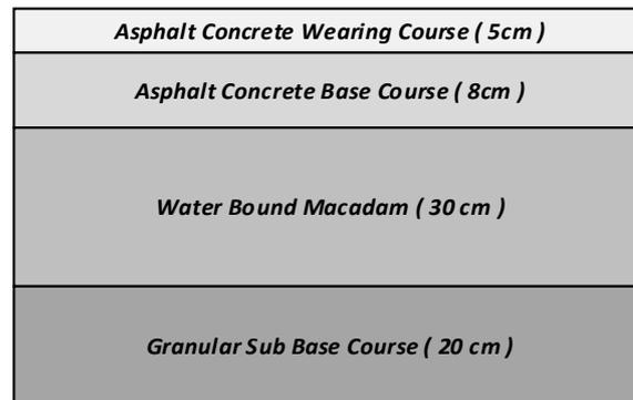
**Figure 1.** Asphalt pavement design.
