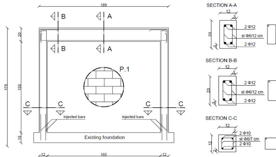
**Figure 10.** Representation of RC frame geometry and elements dimensions.
