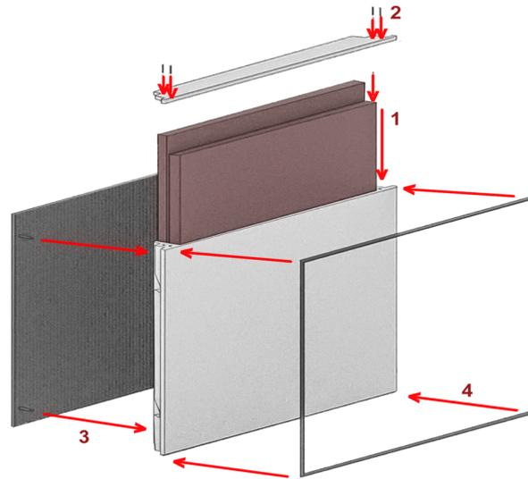
**Figure 9.** Panel module assembly illustration with the assembly steps order marked from 1 to 4.
