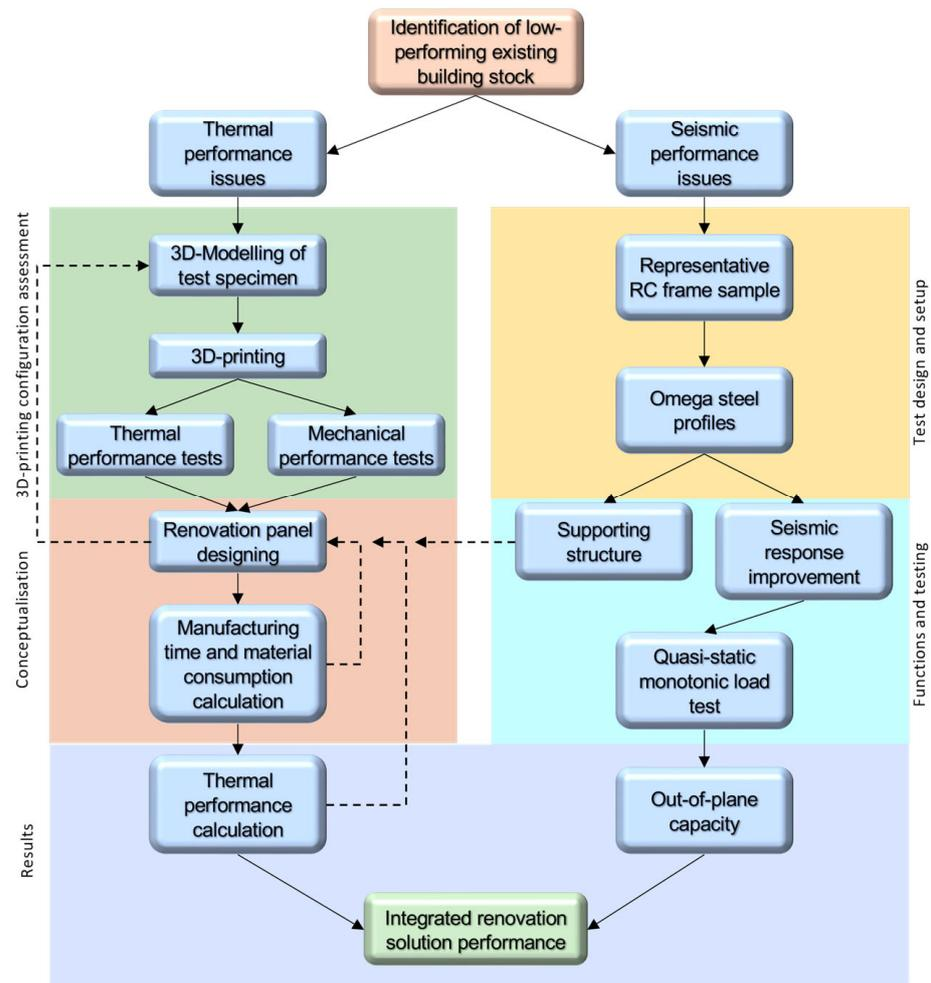
**Figure 1.** Proposed renovation solution development flowchart.
