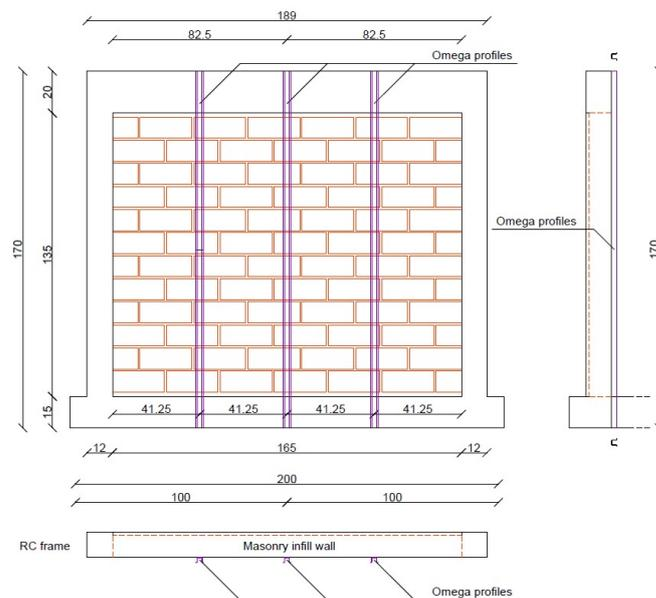
Figure 15. Schematic representation of the reinforced infill wall with omega profiles.
