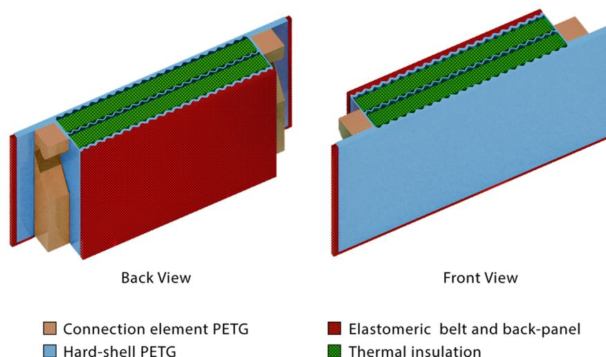
**Figure 3.** Renovation panel parts are illustrated.
