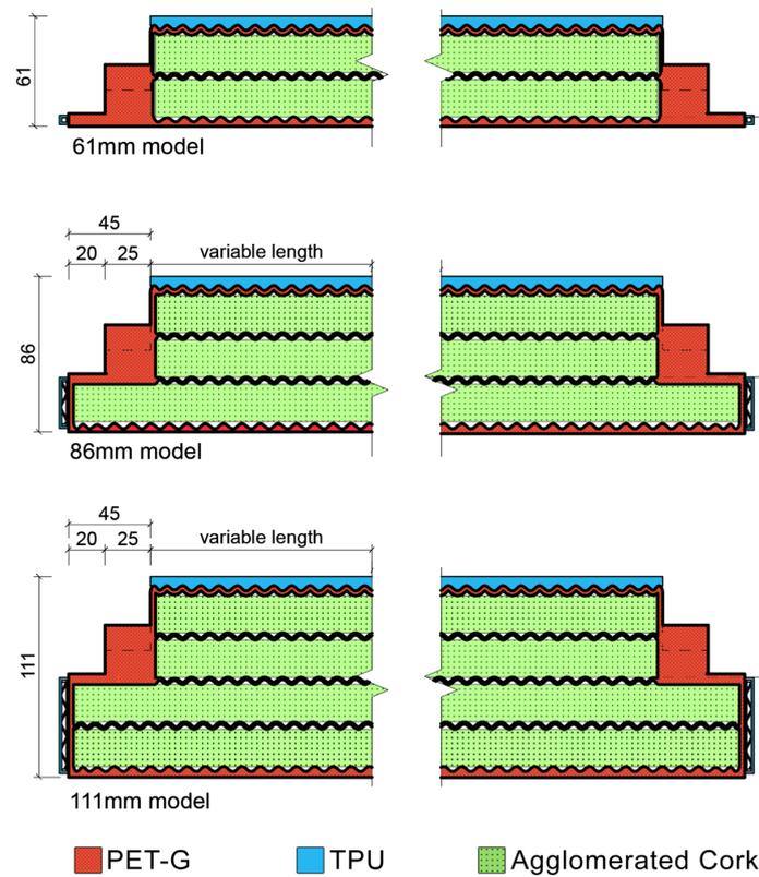
**Figure 6.** 3D-printed building renovation panel sections show the alternative thicknesses and different compositions of the insulation space in between modules in millimetres.
