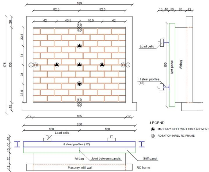
Figure 13. Schematic representation of the test setup layout and the LVDTs location.
