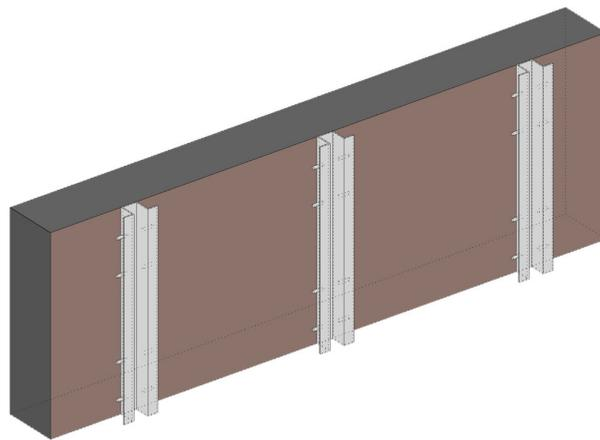
**Figure 2.** A visual representation of the steel structure attached to an infill wall.
