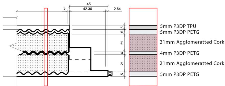
**Figure 22.** 3D-printed panel wall composition for simulation in millimetres.
