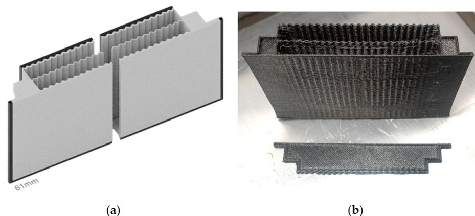
**Figure 7.** (a) Wavy patterns of the renovation panel to avoid structural issues when printing a thin wall with PET-G. (b) The panel prototype displays the wavy pattern of the internal walls.
