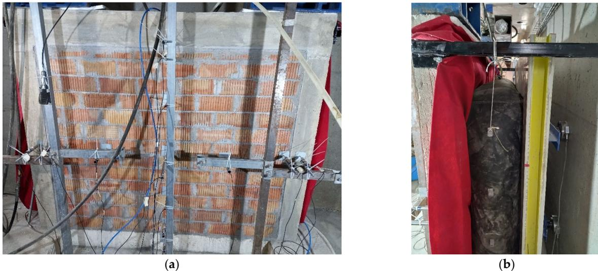
**Figure 12.** URM infill wall testing: (a) Infill wall out-of-plane test setup (front side view); (b) test setup for applying load and contrasting structures (side view).
