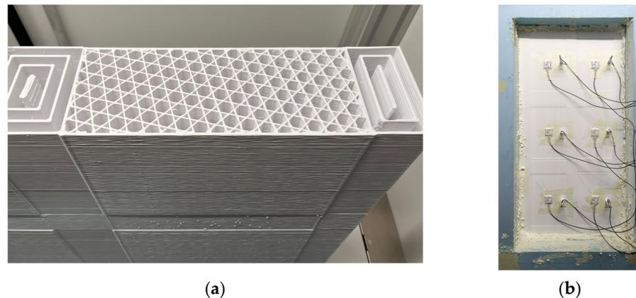
**Figure 21.** (a) 3D-printed 100 mm thick sample of the printing configuration of the PET-G filament with the 25% stars infill. (b) The 3D-printed sample is in the hotbox.
