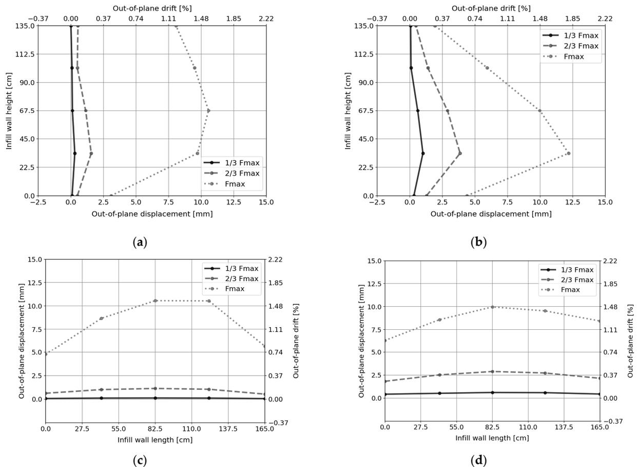
**Figure 20.** Out-of-plane displacement profiles: vertical alignment of (a) URM wall and (b) reinforced infill; horizontal alignment of (c) URM wall and (d) reinforced infill.
