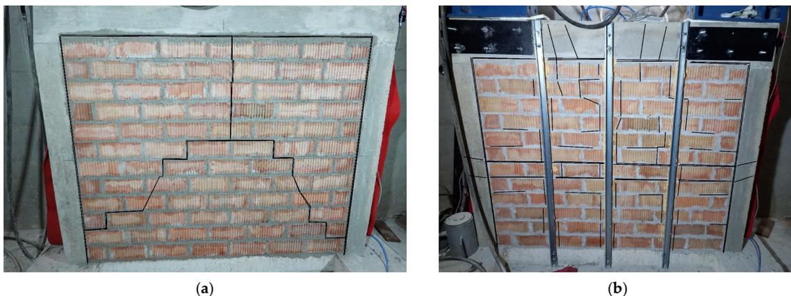
**Figure 18.** Observed damage in the URM infill wall: cracking pattern of (a) URM wall and (b) reinforced infill.
