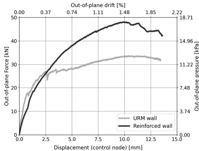
**Figure 17.** Load–displacement curves obtained from experimental testing on URM and reinforced infill walls.
