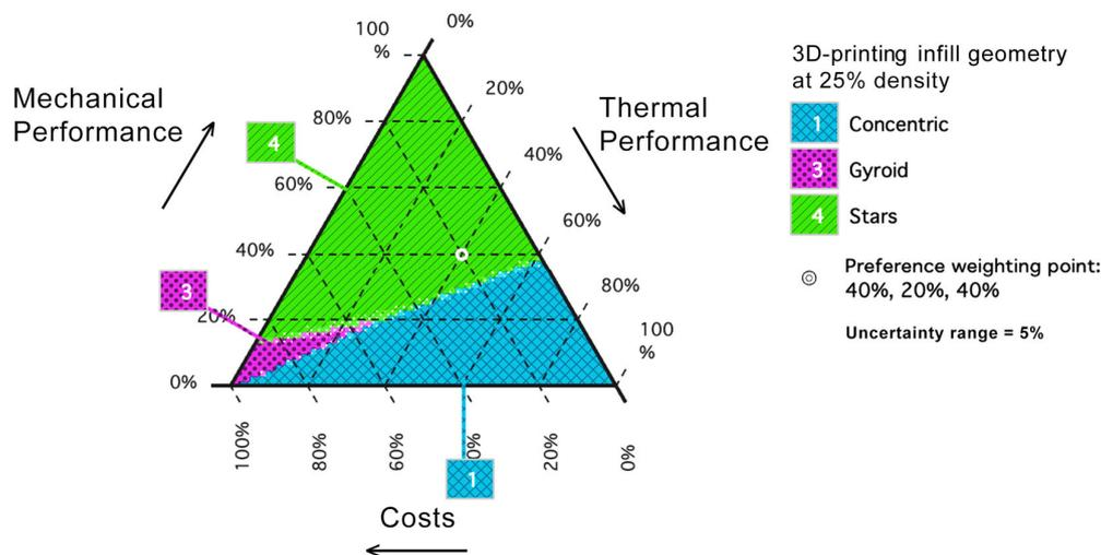
Figure 5. 3D-printing infill geometry optimisation chart, adapted from [18].
