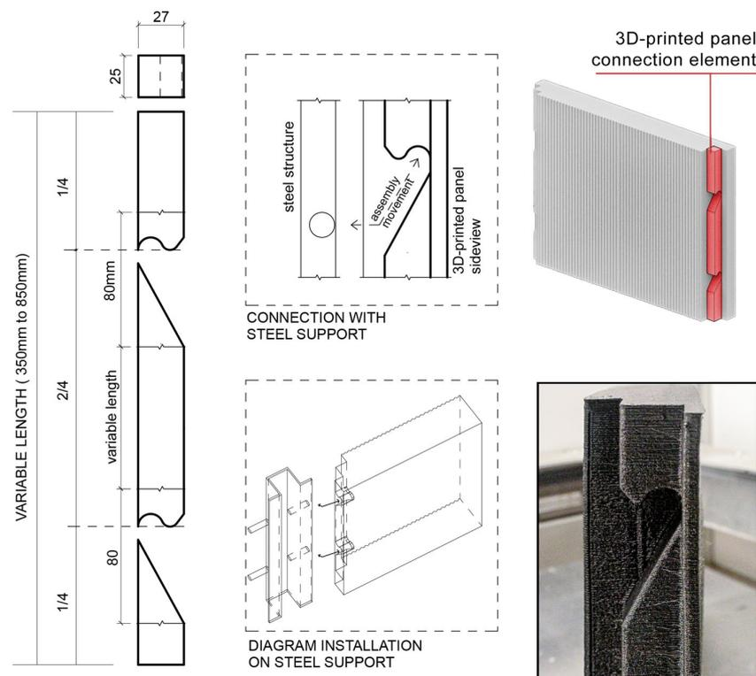
**Figure 4.** 3D-printed building renovation panel connection design to the structural grid in millimetres.
