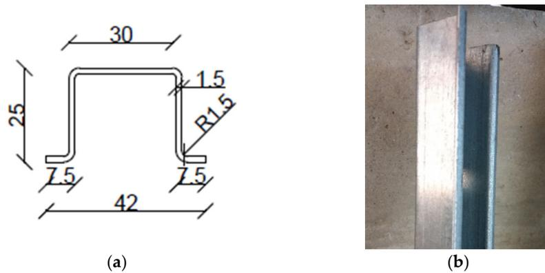
Figure 14. Structural reinforcement: (a) omega section dimensions (half-scale); (b) view of the steel profile.
