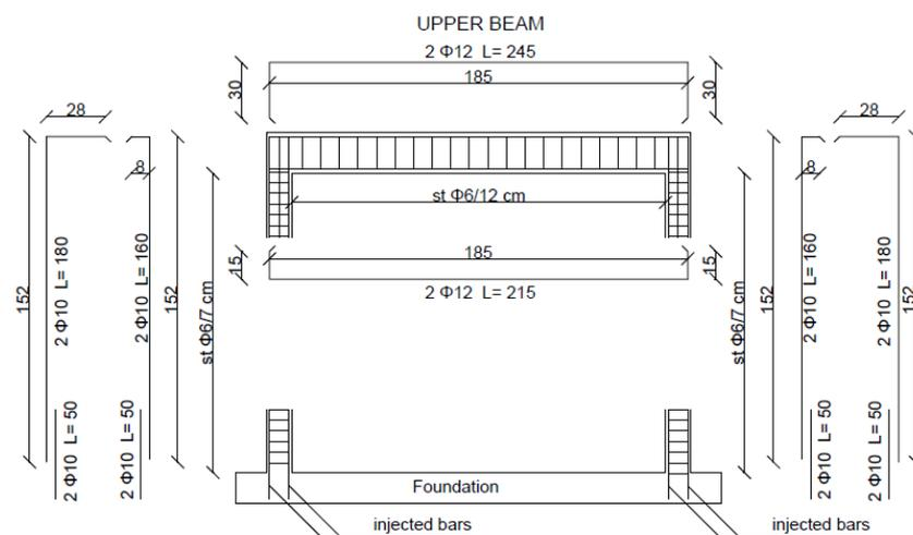
**Figure 11.** RC frame: reinforcement disposition.
