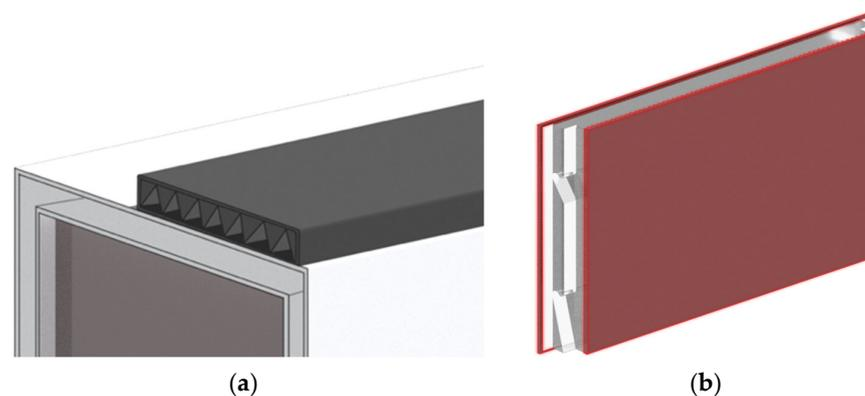
**Figure 8.** (a) Section of the 3D model showing the triangular internal structure of the elastomeric polymer belt. (b) Elastomeric polymer parts, belt, and back panel are highlighted in red.
