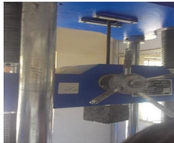
**Figure 7.** Pull-out test.
