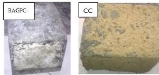
**Figure 10.** BAGPC B4 and CC specimens after 180 days immersed in acid solution.
